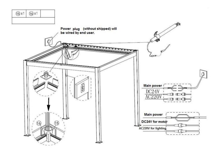
Locate control rod  $\bigcirc$ , Jx 2 (Flat L shape aluminum bar). One is required for each end of the louvers.
