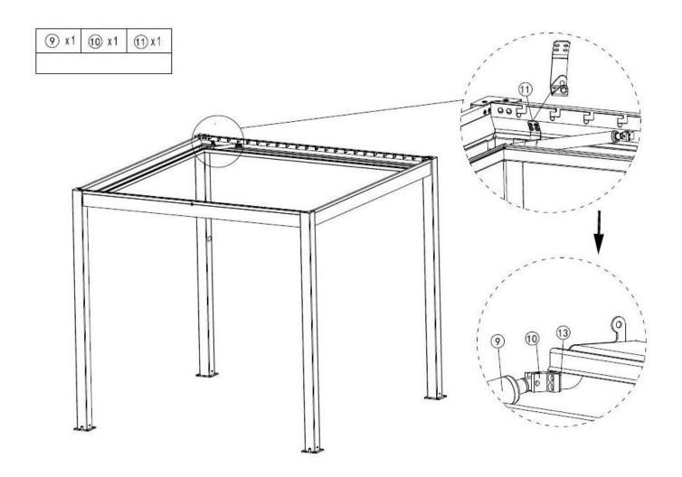
Located holes in centre of beams( ,A and ,B)
